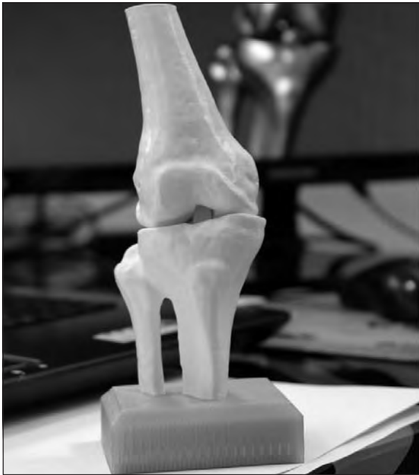
Figura 4. – Realization using 3D printing of a knee model on which the checks (conflicts and distances) were carried out on the movement determined by the insertion between the articular heads with a joint with VRC.
