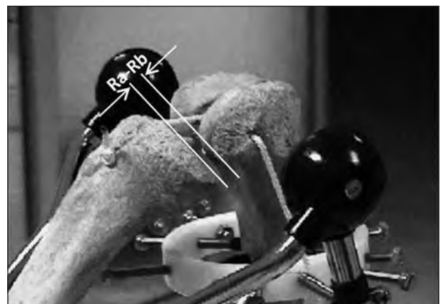
Figura 2. – Distance produced between the articular heads of the knee when it is connected to a mechanical device with fixed center of rotation that does not take account of the distance Ra-Rb determined by the displacement of the centers of rotation in the roto-translatory motion.
